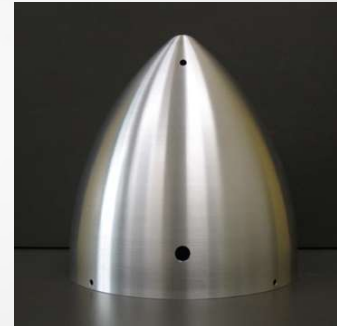
6061-O Alum, Spun Heat Treated to T6
