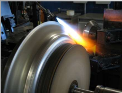
Hot Spinning Titanium Grade 2 & Grade 5
