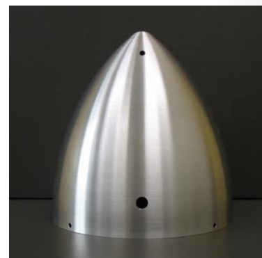
6061-O Alum, Spun Heat Treated to T6
